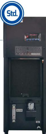
For long-term continuous high-speed operation, a coolant system may be installed to maintain room temperature. The coolant system circulates coolant oil around the spindle bearings to prevent thermal expansion due to the spindle temperature, ensuring high precision machining.
